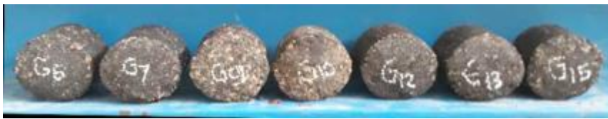
Fig. 8. Deformation of specimens after Marshall testing at flow of 12 mm.
