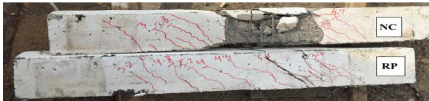
Fig. 11. Show the CC beam ( NC ) and RPC beam ( RP ).
