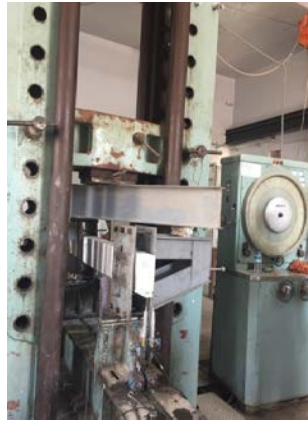
Fig. 8. Show the LVDT, steel arms and machine test.
