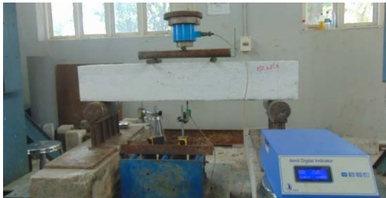
Fig. 6. Test setup for testing flexural behaviour of RCC beam.
