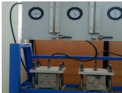
Fig. 4. Water permeability test.
