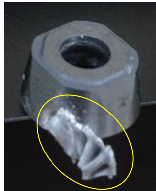
Fig. 6. Evolution of built-up at cutting speed of 600 m/min.
