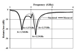
(a)  $|S_{II}|$  characteristics for proposed Antenna-II when  $L_i = 35$  mm.
