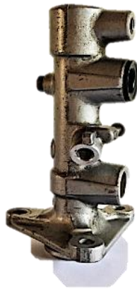
Fig. 2. A clutch master cylinder utilized for a photogrammetry model as a case study.
