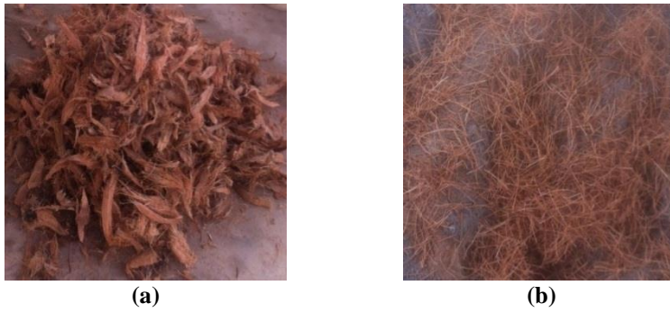
Fig. 2. Removed coir fibre: (a) Before pre-treatment and sizing, (b) After pre-treatment and cutting to average 40 mm length and diameter of 3.6 µm.
