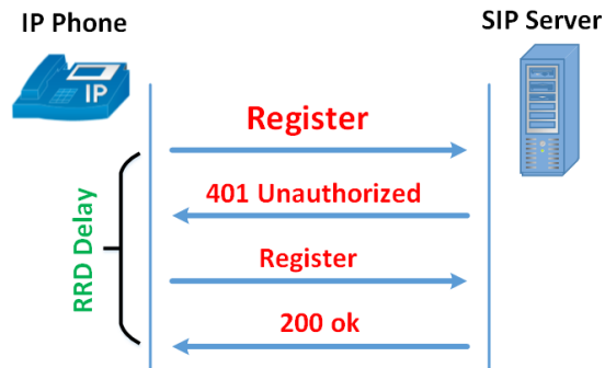
Fig. 1. SIP client registration process.
