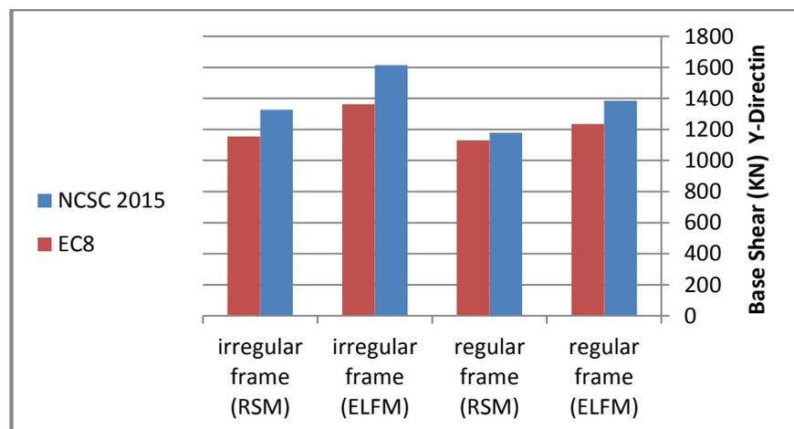
Fig. 10. Total base shear in *y*-direction.
