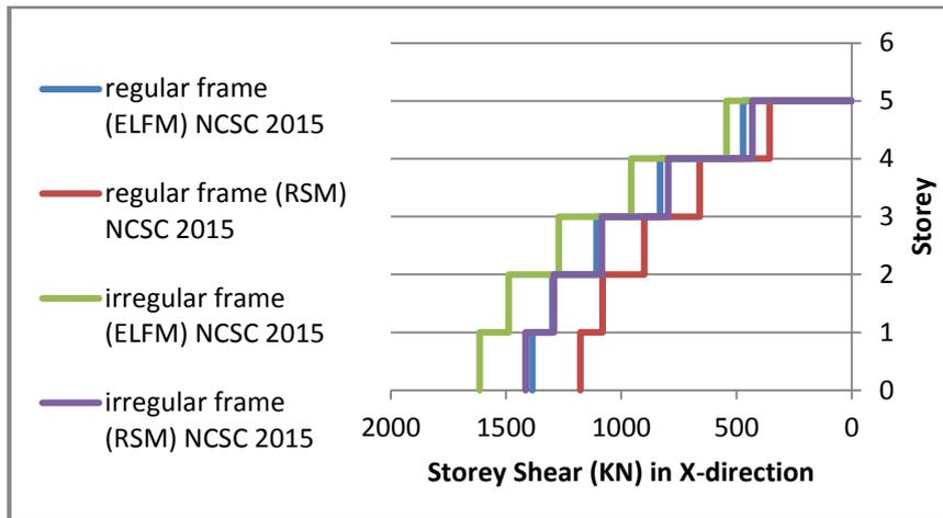
Fig. 11. Storey shear according to NCSC 2015 in  $x$ -direction.
