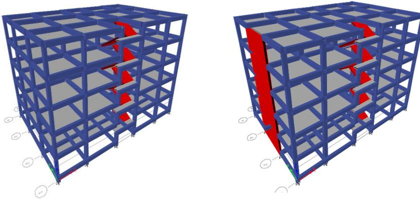
**Fig. 8. View of 3D model of G+4 storey regular and irregular RC frame.**
