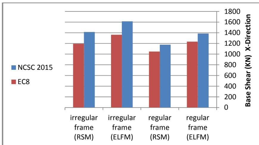
Fig. 9. Total base shear in *x*-direction.
