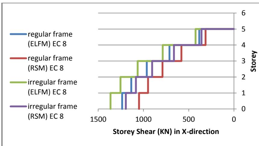
Fig. 12. Storey shear according to EC 8 in  $x$ -direction
