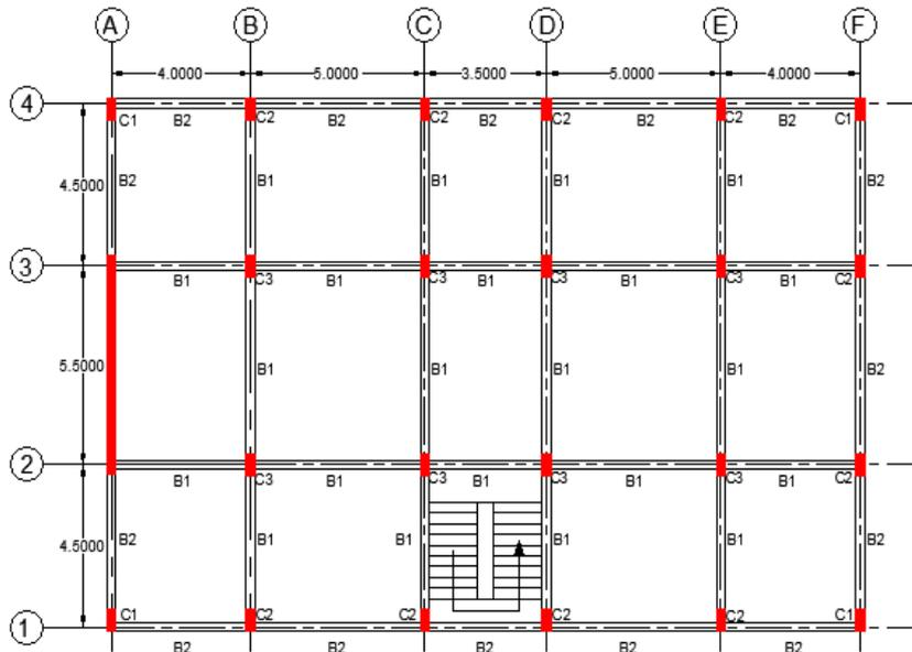
Fig. 7(b). Floor plan for G+4 storey irregular RC frame.
