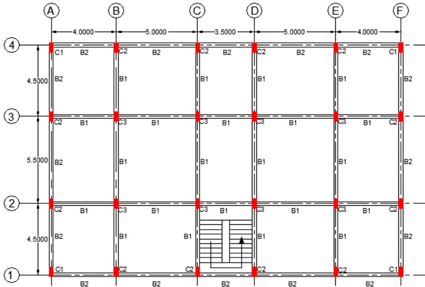
Fig. 7(a). Floor plan for G+4 storey regular RC frame.
