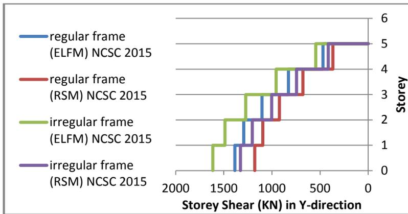
Fig. 13. Storey shear according to NCSC 2015 in y-direction.
