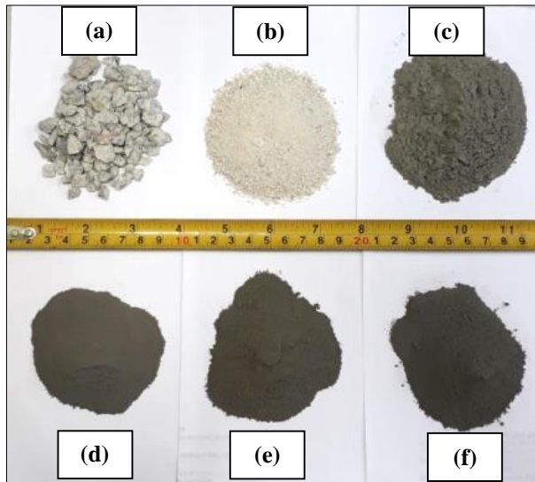
Fig. 2. Materials used in this study, (a) coarse aggregate, (b) sand, (c) OPC, (d) CBA with 20 hours grinding, (e) CBA with 30 hours grinding, and (f) CBA with 40 hours grinding.
