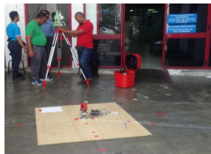
Fig. 13. JUPEM observed the difference of Qibla direction marked by prototype.
