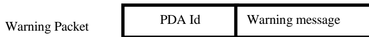
Fig. 2. Packet delivered to PDA by node to inform about RF link failure.
