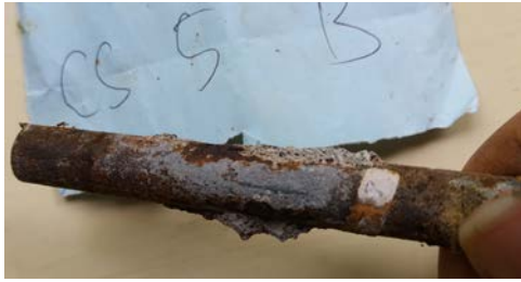
Fig. 5. Corrosion product on steel bar.
