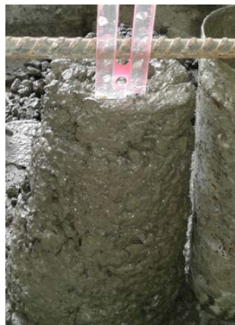
Fig. 7. Slump of conventional concrete.
