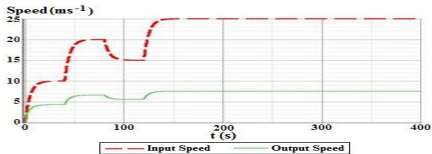
Fig. 8. Input and output speeds of the vehicle with disturbance.
