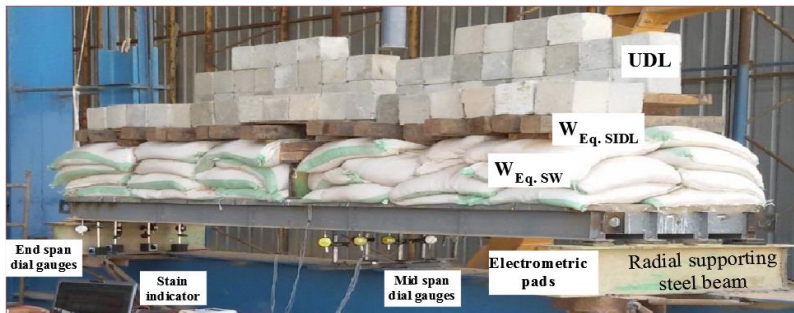
Fig. 6. Test rig elements.
