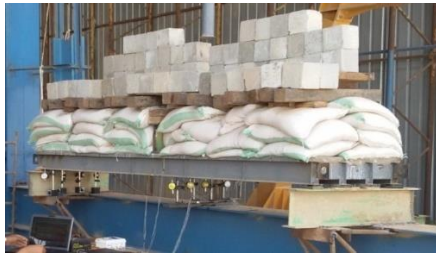
Fig. 10. Equivalent SW+SIDL + Lane load.
