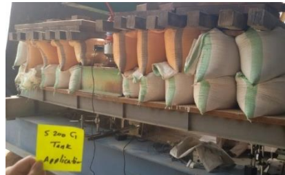
Fig. 11. Equivalent SW+SIDL+ Tank.
