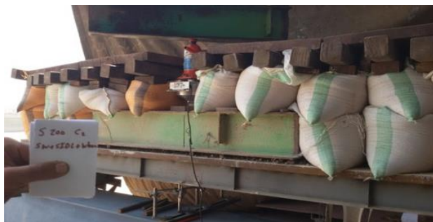
Fig. 12. Equivalent SW+SIDL+ wheel loads.
