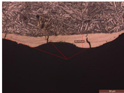
Fig. 4. Micro-structure representing surface roughness R_a (SR) and RLT .
