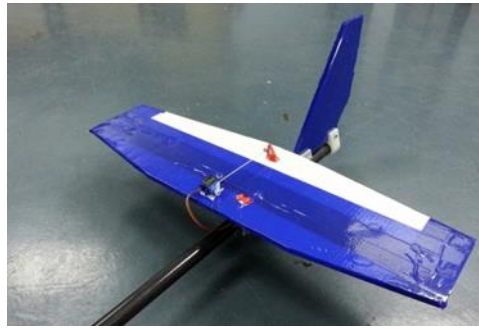
Fig. 3. All-moving horizontal stabilizer with trailing edge elevator.
