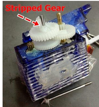
Fig. 1. Faulty servo actuator.
