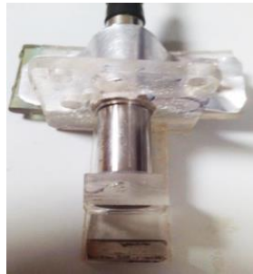
Fig. 4. Transducer probe with reflector and buffer rod.
