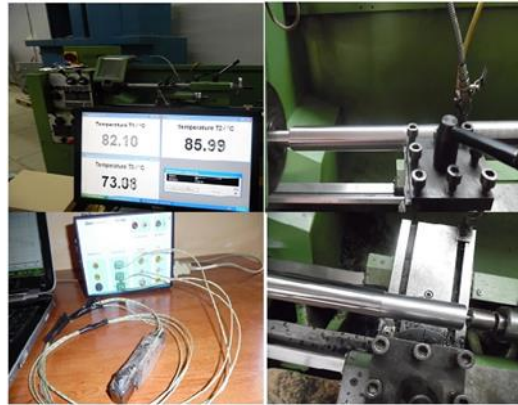
Fig. 1. The experimental setup used for the temperature measurements.
