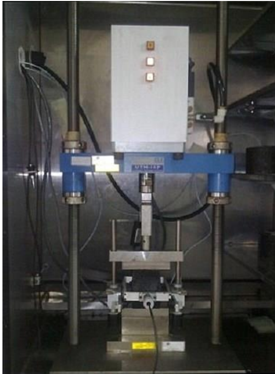
Fig. 2. UTM 14P for resilient modulus test.
