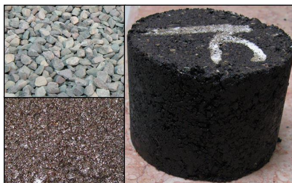
Fig. 1. Compacted asphalt mixture specimens.
