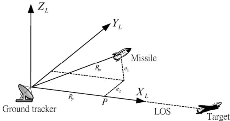
Fig. 2. Definition of tracking error [13].
