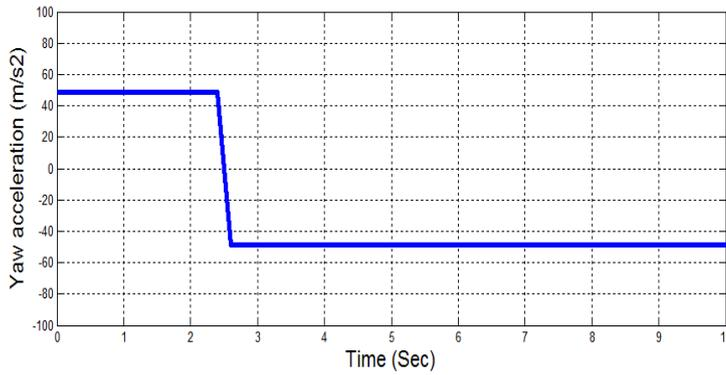
Fig. 5. Yaw acceleration command.
