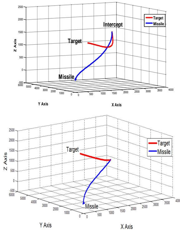
**Fig. 8. Engagement responses of Clos missile guidance law, (a) Feedback linearization guidance, (b) Fuzzy adaptive guidance.**
