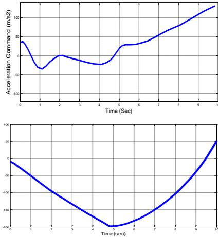
**Fig. 9. Acceleration command  $a_{zc}$ , (a) Feedback linearization guidance, (b) Fuzzy adaptive guidance.**
