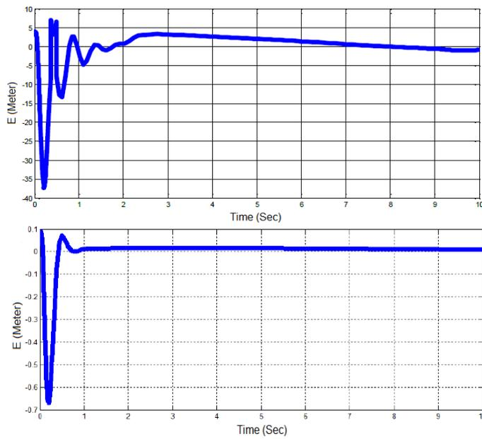
**Fig. 7. Tracking error  $e_1$ , obtained by applying (a) feedback linearization, and (b) fuzzy adaptive design.**
