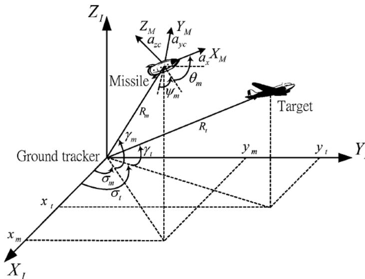
**Fig. 1. Diagram of the missile and target tracking in 3-D [13].**
