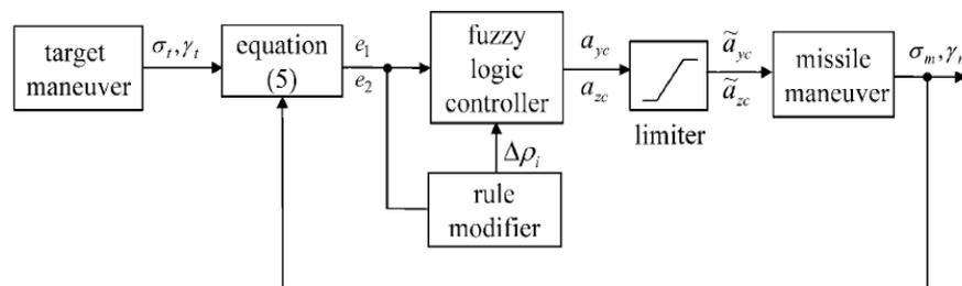
Fig. 3. Guidance system for CLOS guidance law.
