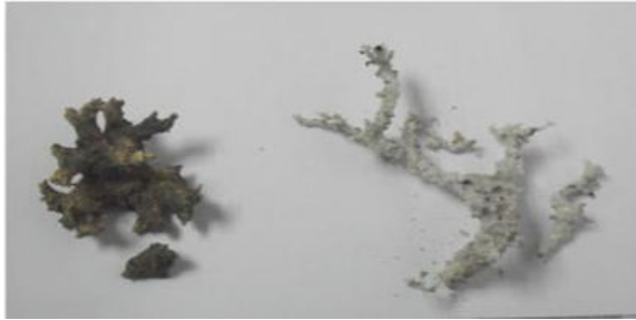
Fig. 14. Fulgurites Formed in Bentonite (left) and Sand (right) [5].
