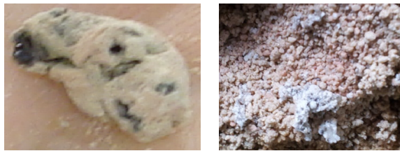
Fig. 13. Fulgurites Formed in Bentonite (left) and in Wet Sand (right).
