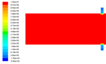
Fig. 6. Static pressure contours for double outlet ports actuator.
