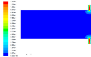
Fig. 7. Velocity contours for double outlet ports actuator.
