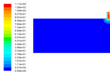
Fig. 4. Velocity contours for one outlet actuator.
