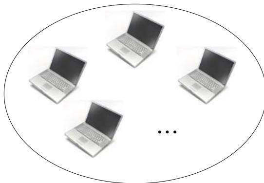
Fig. 3. The single-BSS ad hoc network topology.
