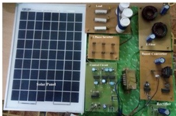
Fig. 10. Prototype hardware model- Z-source inverter for solar energy system.
