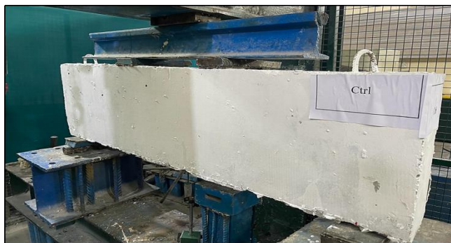
Fig. 4. Deep beam specimen under test machine.
