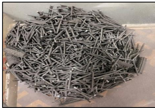
Fig. 2. Recycled steel fibre extracted from end life use tyres.
