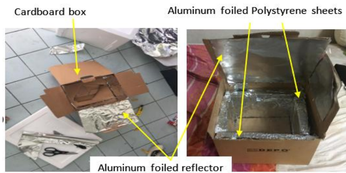
Fig. 3. Model fabrication of the box-type solar cooker.
