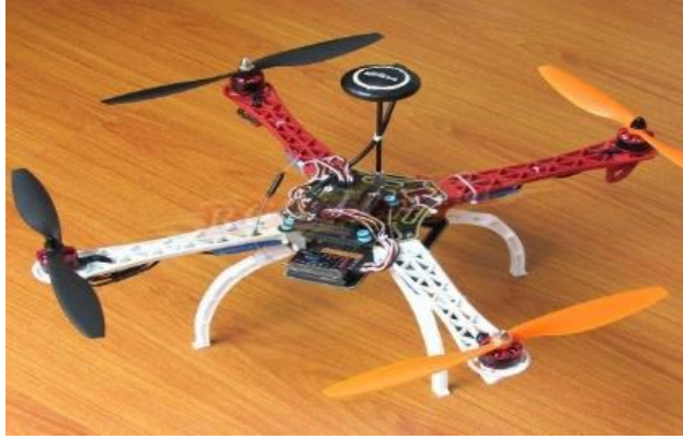
Fig. 2. Fabricated UAV with control system.
