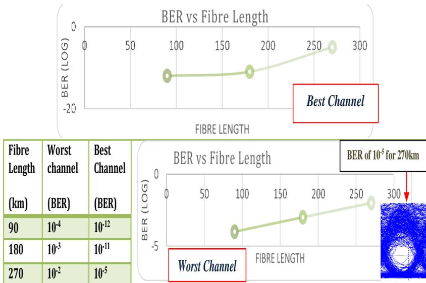
Fig. 9. BER values for 16 Channel WDM NRZ-OOK (Bit Rate: 40 Gb/s).
