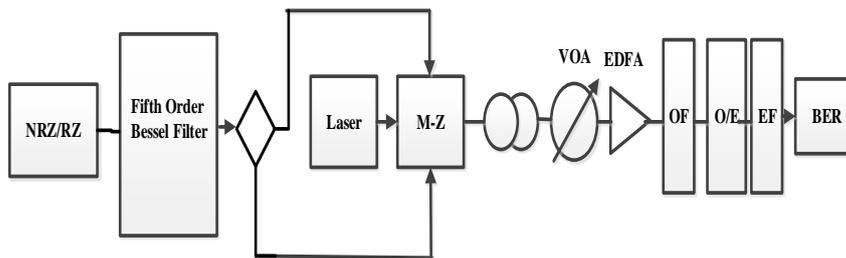
**Fig. 4. NRZ-OOK and RZ-OOK simulation set-up.**
