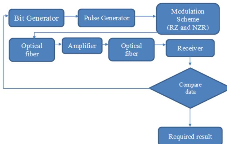
Fig. 3. Process flow of the methodology implemented.
