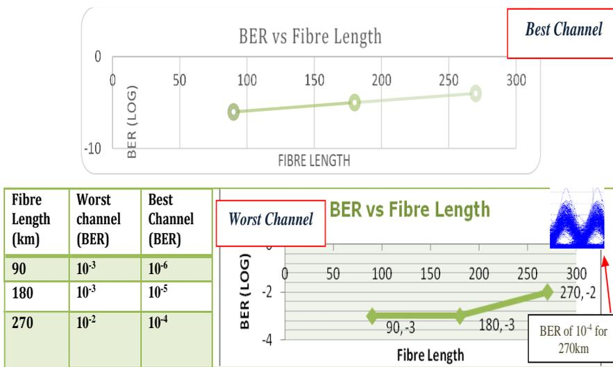
Fig. 11. BER values for 16 Channel WDM RZ-OOK (Bit Rate~ 40 Gb/s).
