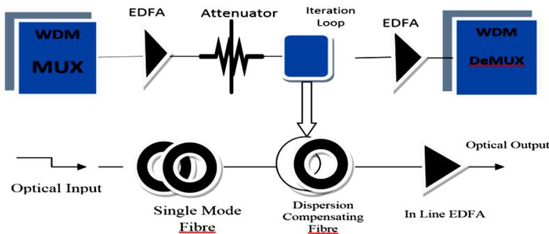
**Fig. 5. Transmission link set-up.**
