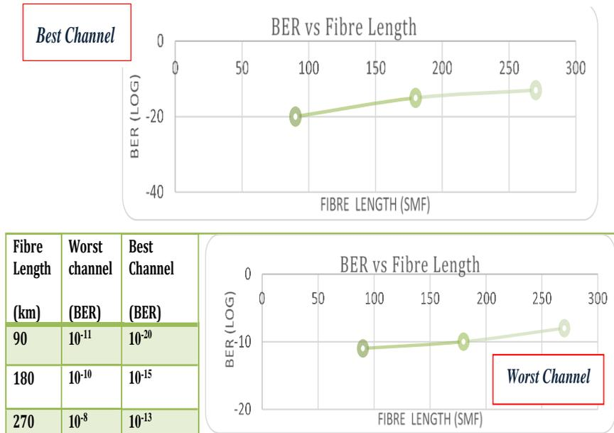
Fig. 8. BER values for 4 Channel WDM NRZ-OOK (Bit Rate~ 40 Gb/s).
