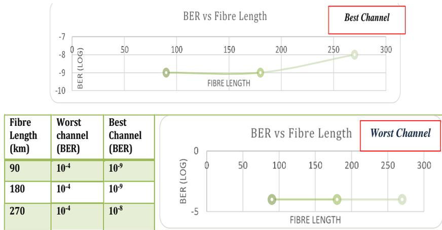
Fig. 10. BER values for 4 Channel WDM RZ-OOK (Bit Rate~ 40 Gb/s).
