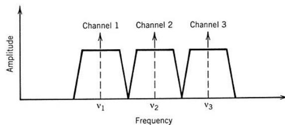
Fig. 2. Wavelength division multiplexing [9].
