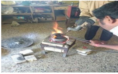
(a) CF and SiC poured aluminium cast
