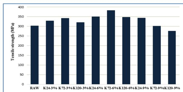
**Fig. 1. Effect of NaHCO<sub>3</sub> on tensile strength of KF.**
