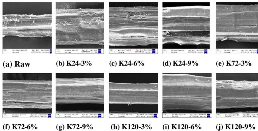
Fig. 3. SEM micrograph of raw and treated fibres.
