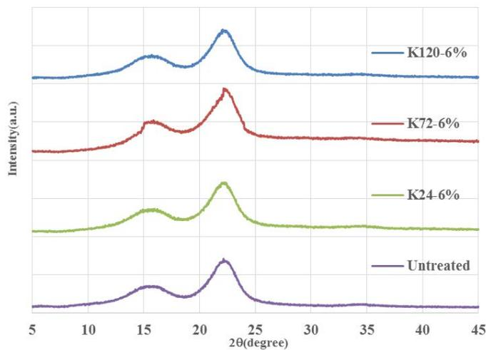
Fig. 2. XRD diffractograms of raw and alkali treated KF bundles.
