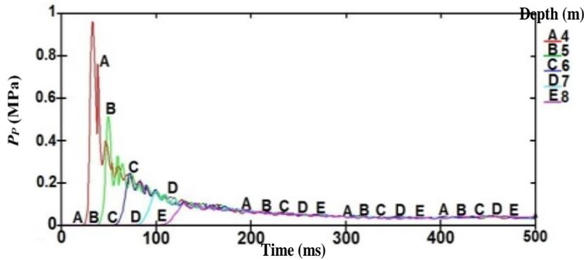
Fig. 2. Time histories of blast peak pressure into soil at different depths.
