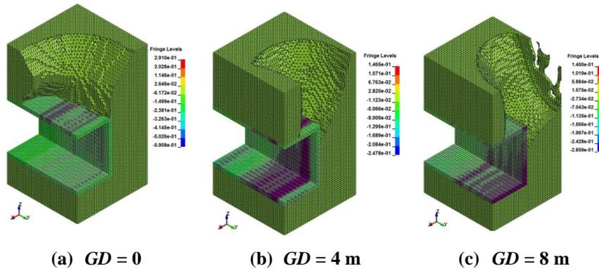
**Fig. 8. Lateral displacement contours of tunnel at different blast ground distance.**
