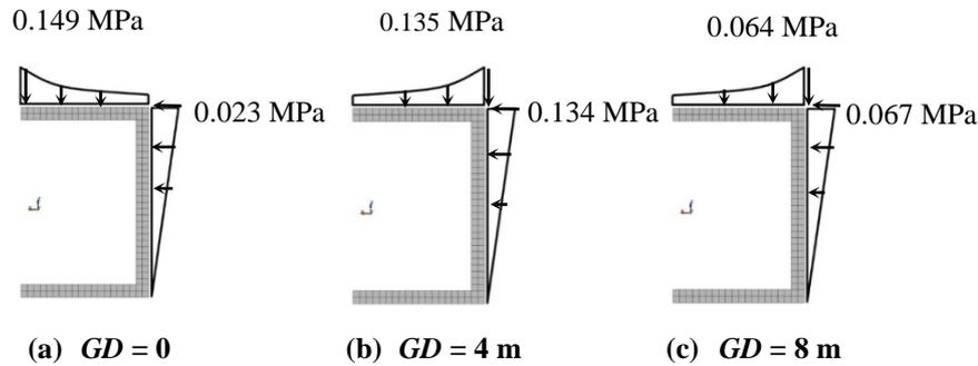
**Fig. 6. Reflected pressure (MPa) of tunnel at different blast ground distance.**
