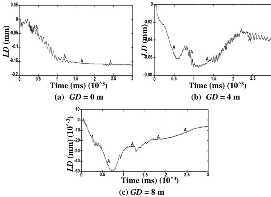
**Fig. 7. Time histories of lateral displacement for tunnel center at various blast ground distance.**
