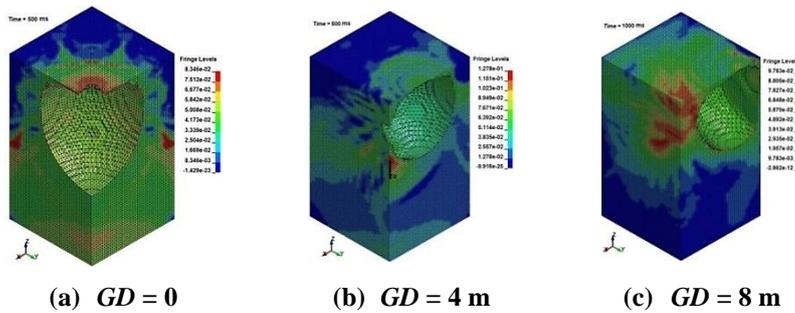
Fig. 5. Propagation of blast waves into soil at various ground distance.
