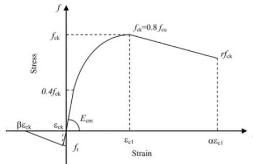
**Fig. 3. Stress-strain curve for the concrete material.**
