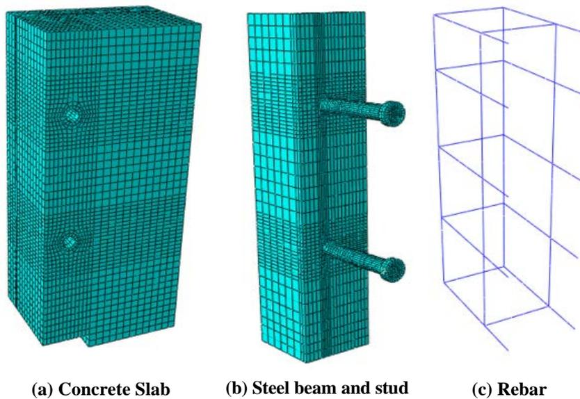
**Fig. 1. Finite element type and mesh.**
