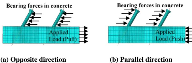
**Fig. 7. Bearing forces in concrete in the direction of the applied force.**
