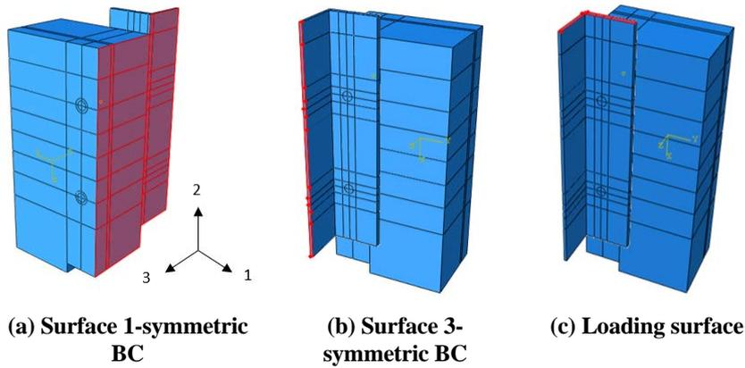
**Fig. 2. Boundary condition and loading surfaces.**
