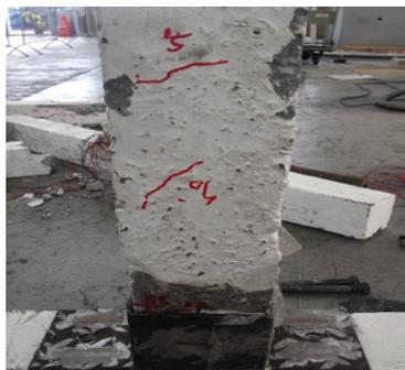
Fig. 14. First and second crack at hidden corbel connection.
