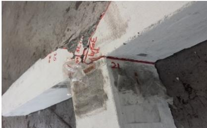
Fig. 12. First crack of monolithic.
