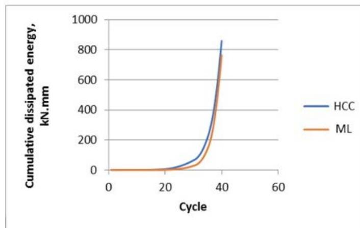
Fig. 8. Cumulative energy dissipation curves of the two specimens.
