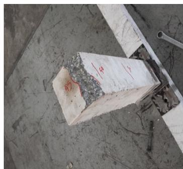
Fig. 15. Spalling of concrete of the beam of hidden corbel.
