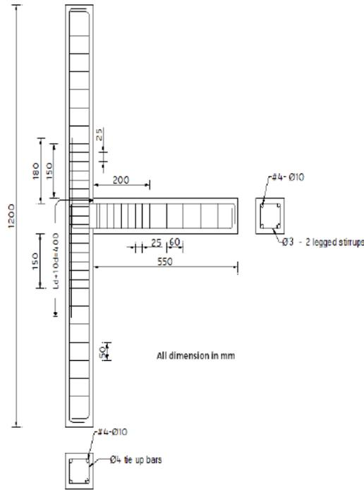
**Fig. 1. Details of monolithic.**
