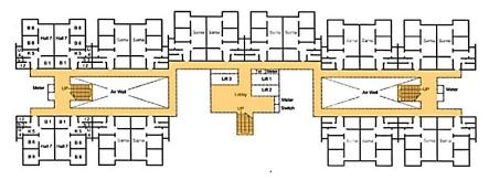
Fig. 1. Typical plan for an 18-storey low-cost flat with yellow highlights indicating the transitional spaces.
