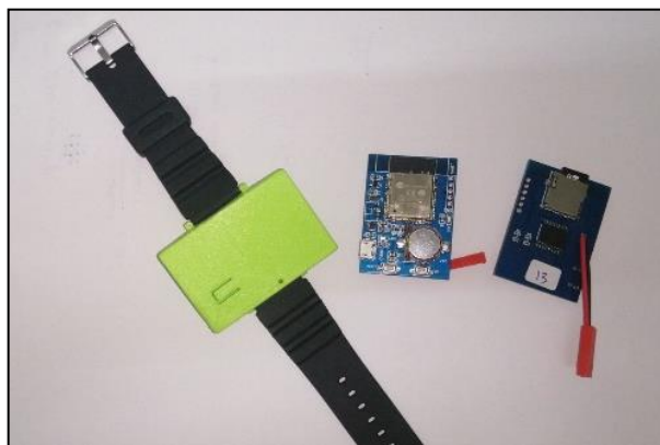
Fig. 21. Final hardware and customize PCB (front & back).
