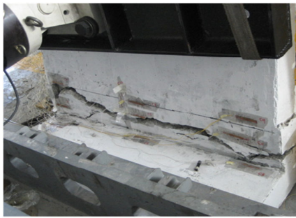
Fig. 11. EIWC1 Specimen at Failure.
