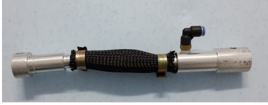
Fig. 1. McKibben Pneumatic Artificial Muscle.
