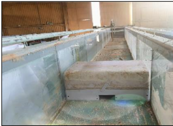
Fig. 2. The broad-crested weir model with an orifice (rectangular shape).
