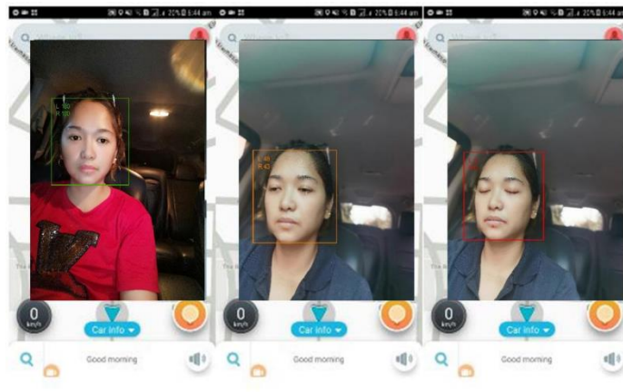
Fig. 6. Detection of faces during both daytime and nighttime employed by car drivers.
