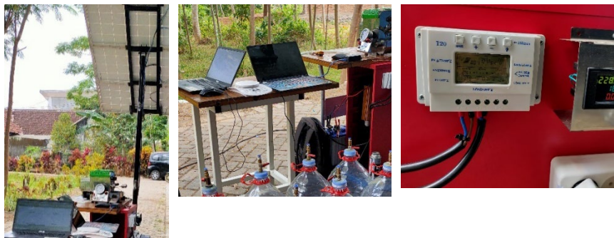
Fig. 4. Solar panel (left), coffee roaster machine (middle), AC power meter (black, right), DC power meter (white, right).
