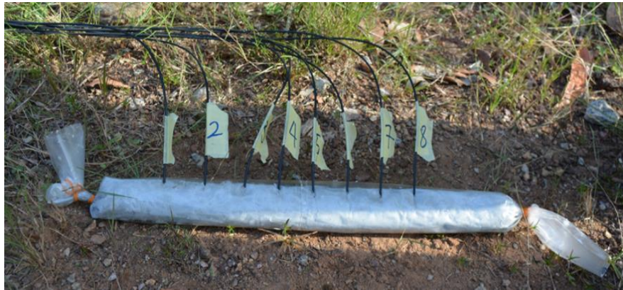
Fig. 8. Detonation velocity testing using fiber optic cables [2].
