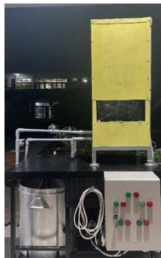
Fig. 2. Implementation of the Cooling Tower prototype hardware.
