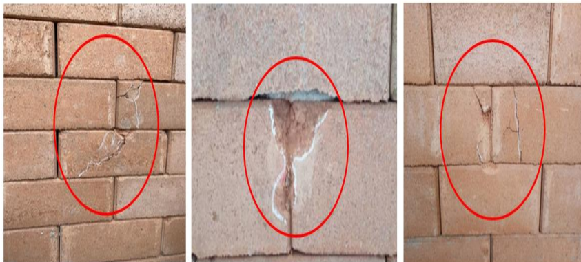
(a) Unreinforced wall. (b) Steel-reinforced wall. (c) Bamboo-reinforced wall.
