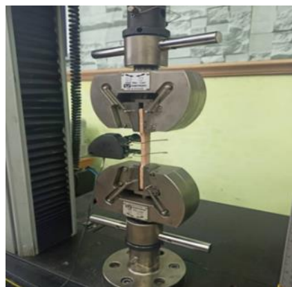
Fig. 10. Tensile strength test of bamboo using Instron UTM.
