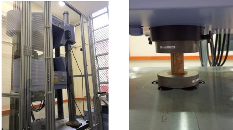
Fig. 9. Compression test of bamboo using Shimadzu UTM.
