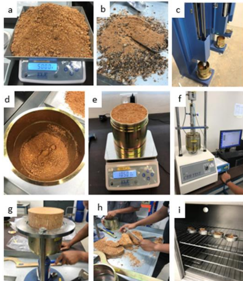
Fig. 4. The CBR test procedures according to MS1056:PART4:2005.
