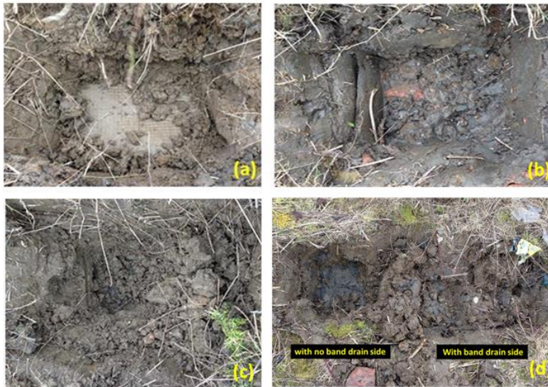
Fig. 4. (a) Panel 1- cusped core GD, (b) Panel 2 (Control panel) - without any geosynthetic drain, (c) Panel 3- non-woven needle punched geotextile GD and (d) Panel 4- GD with band drains and with no band drain side.
