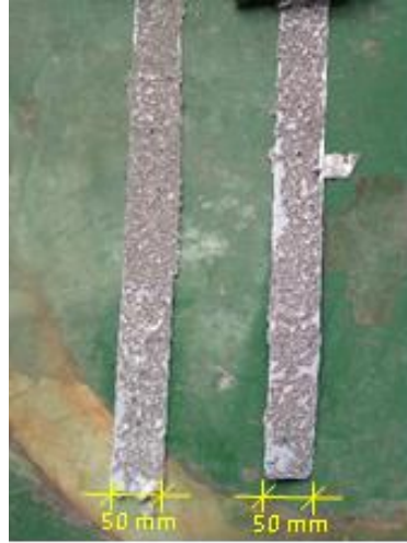
Fig. 6. Cold-formed steel plate as strengthening.
