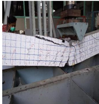
Fig. 4. BU - B0 crack patterns.
