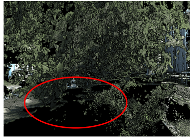
Fig. 5. The road beneath the vegetation was not captured by UAV LiDAR between STA 0+100 and STA 0+150.
