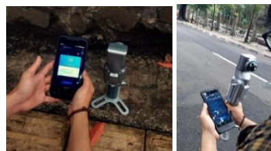
Fig. 7. Data collection process using SLAM scanner.
