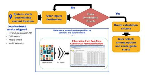
Fig. 2. High level flow chart of path planning process with RT-CTFS as standardized database.
