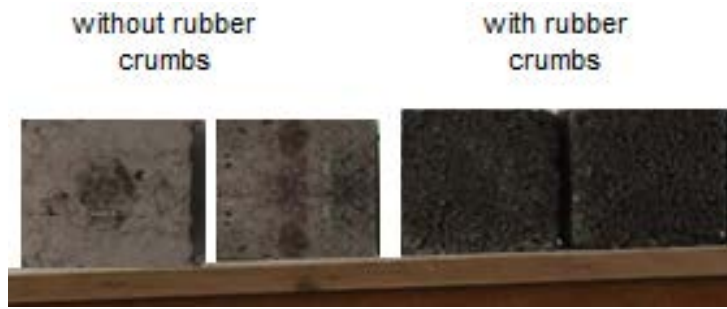
Fig. 5. The appearance of fine aggregate replacement with rubber crumbs concrete specimens.
